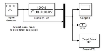
The tutorial shows how to use the Simulink Real-Time software, the Simulink Coder environment, and a third-party compiler. It describes how to create a real-time application from xpc\_osc3, build and download it, and execute it on the target computer.
